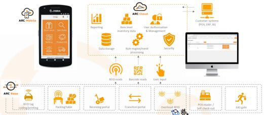
To deal with data volumes typically generated by fixed (overhead) readers, ARC Base is usually deployed on a (VM) server at the store. ARC Cloud runs on M&A's VPC at AWS and ARC Mobile is a native client available both for iOS and Android.
