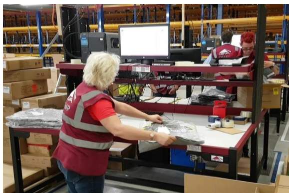
Example: RFID packing table for outbound at Ceva Logistics UniQlo EDC in Oud-Gastel, Netherlands.
