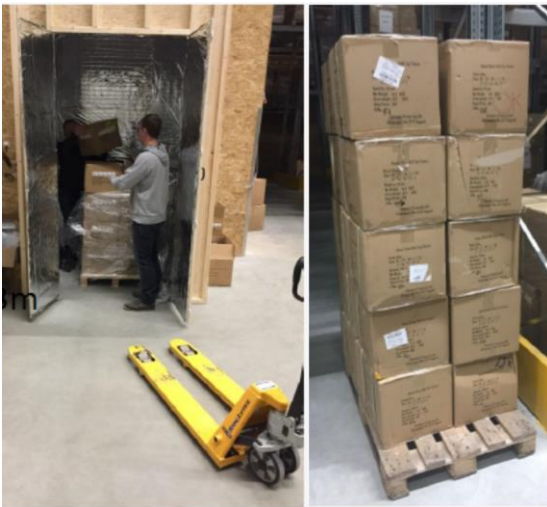
Example: low-cost full pallet RFID chamber reading up to 1.200 items in less than 10 seconds.
